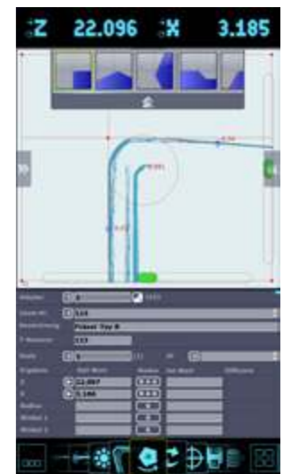
»cris360°« (circular response image sampling) software function for measuring the maximum tool contour
