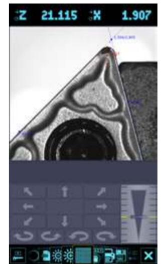
Cutting edge inspection with dimmable light on the camera
