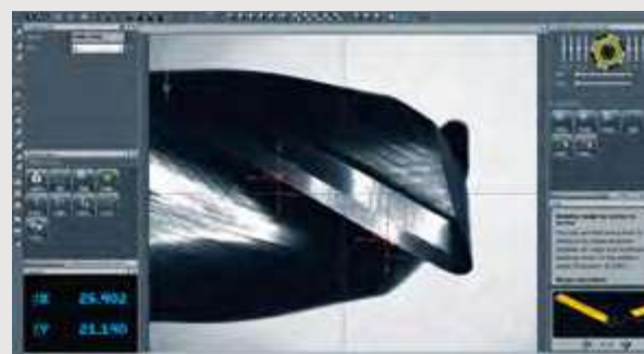
Determination of chamfer width and spiral angle.
