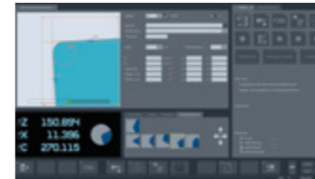
Simple manual measurement with automatic cutting-edge shape identification, without generating data and specification of nominal values.
