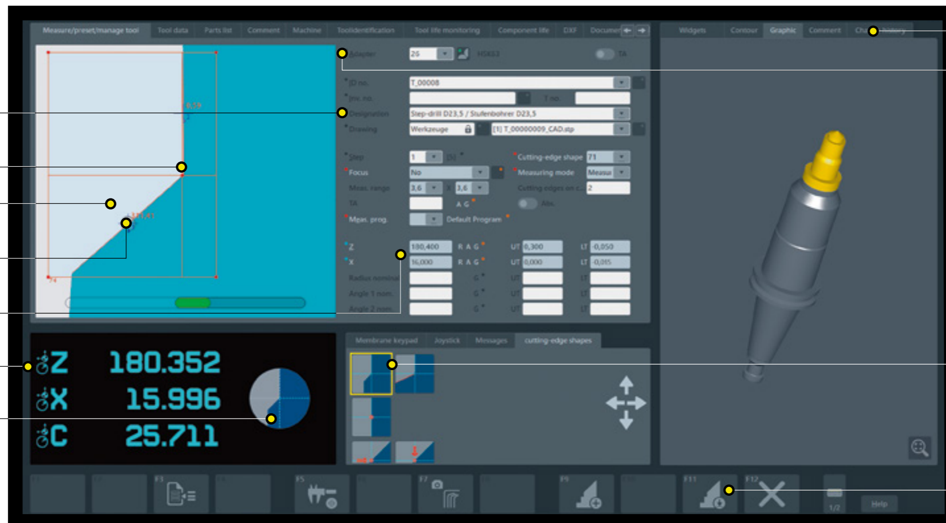
Comprehensive selection of measuring programs in »pilot 4.0« with photo realistic input dialog for simple operation and reliable nominal dimension specification.
