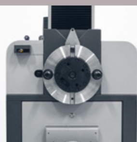
High-precision spindle and tool holding fixture with power clamping 20,000 N, universal interface and tool post with loading safety
