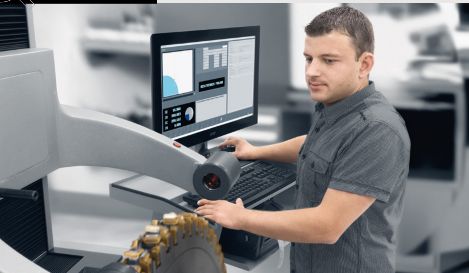
High-precision spindle and tool holding fixture with power clamping 20,000 N, universal interface and tool post with loading safety
