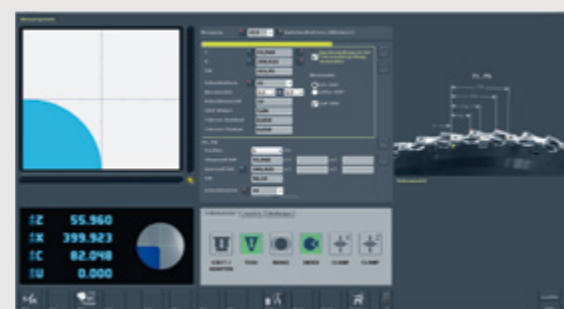
Measuring program for calculating the average values of circumferential cutting edges at several cutting edge stages.
