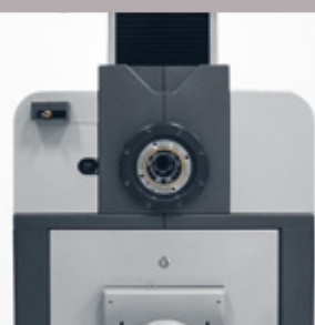
High-precision spindle and tool holding fixture with power clamping 20,000 N, universal interface and tool post with loading safety
