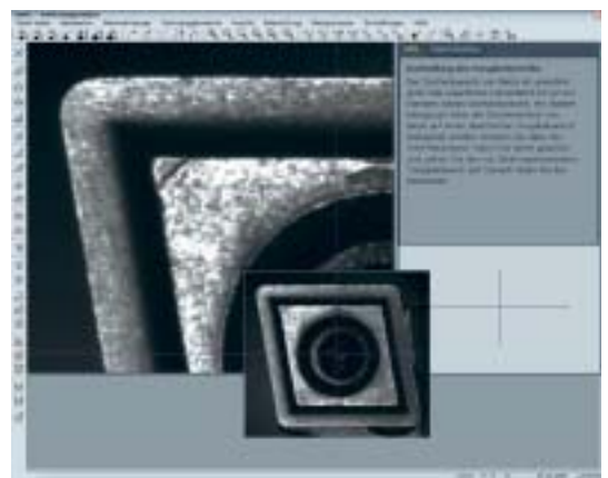
Incident light measurement at chip space and inspection with »metis«, 1:1 magnification and zoom.
