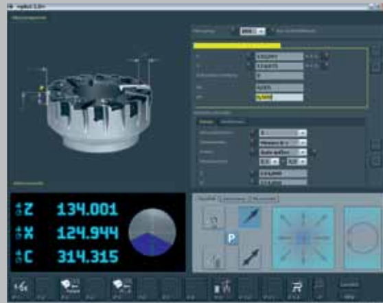
Input dialog »FORED«, example measuring program "Milling cutter with roughing and finishing cutting edges"
