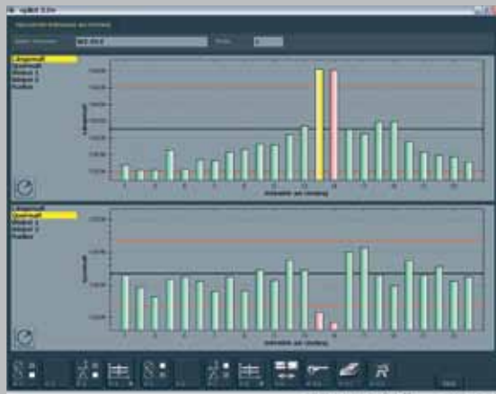
Diagram "Largest cutting edge" with tolerance range and function cutting edge correction
