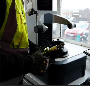
DoorCo invested in a ZOLLER smile 420 tool presetter from ZOLLER UK, enabling them to unlock significant production capacity.
