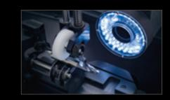
The **»pomBasic«** inspection machine checks tools on up to 70 tool parameters in a matter of seconds. Insert, align, measure.
