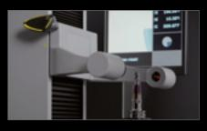
By scanning the ZOLLER **»idChip«** on the presetting and measuring machine, the tool data is called up directly and the measurement sequence can start.
