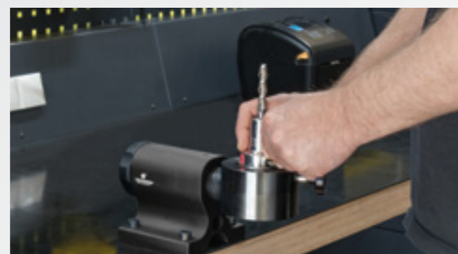
Tool assembly device for secure tool assembly
