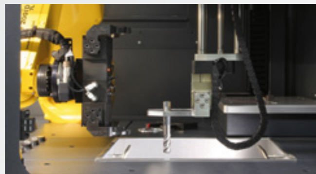
Cleaning of the tool cutting edges in the ultrasonic bath
